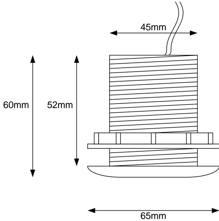
Max hull thickness 37mm
