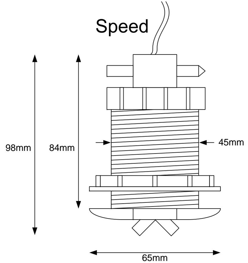
Max hull thickness 26mm
